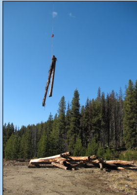
Helicopter long lining logs to the Sherlock site.
